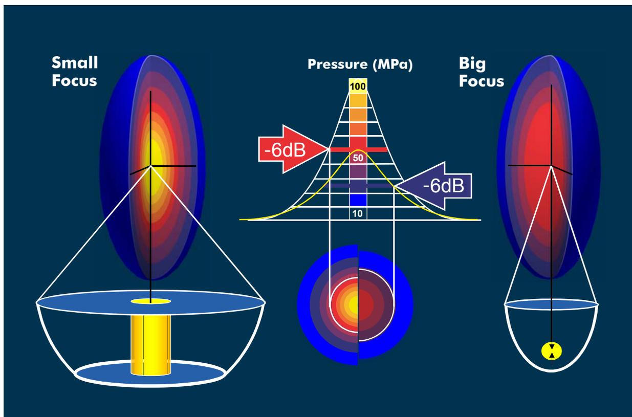
Due to physics a small focus is only possible with large apertures and generators with small apertures are only capable to form a big focus. It must be emphasized again that this holds true independent from the energy content and thus from the expected medical efficiency.
